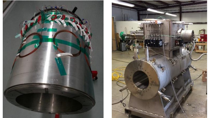
Figure 3: Picture on the left show manufactured singlet with aluminum containment ring. Picture on the right shows the cryostat housing the three singlets
