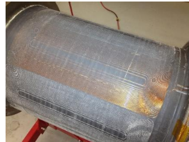
Figure 4: Coil support cylinder with machined grooves for a SSC CCmT coil. Grooves in lighter shade already have conductors placed in them.
