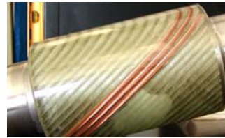
Figure 5. A few turns of epoxy impregnated coil, with a Lexan cover, show typical turn geometry. Insulation is provided by the web of the coil support grooves and the epoxy impregnation.
