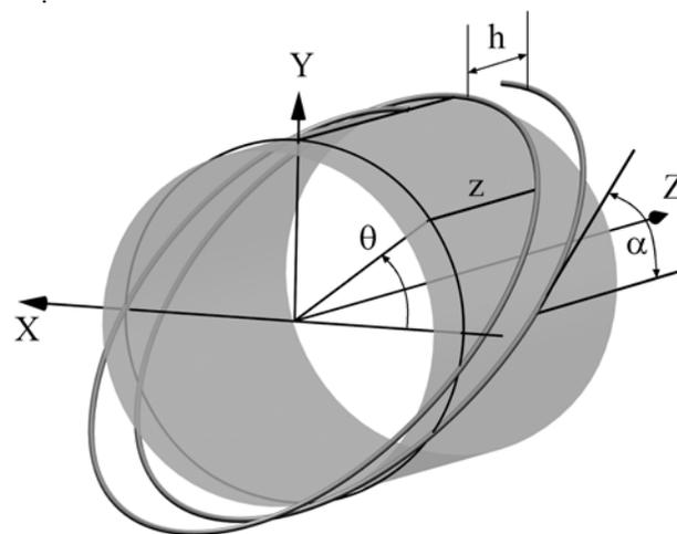
Fig. 2. Coordinates of tilted helical loops with modulation  $n=1$  (dipole)
