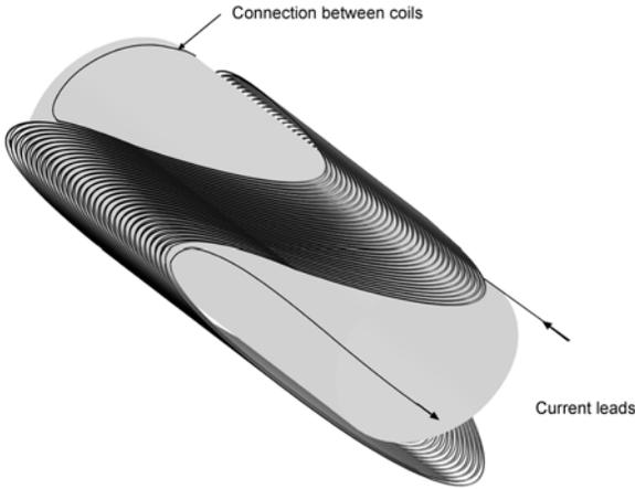
Fig. 4. Coil arrangement for a double-helix quadrupole (DHQ). Partial length coils are shown, to illustrate both lead and return ends of winding.
