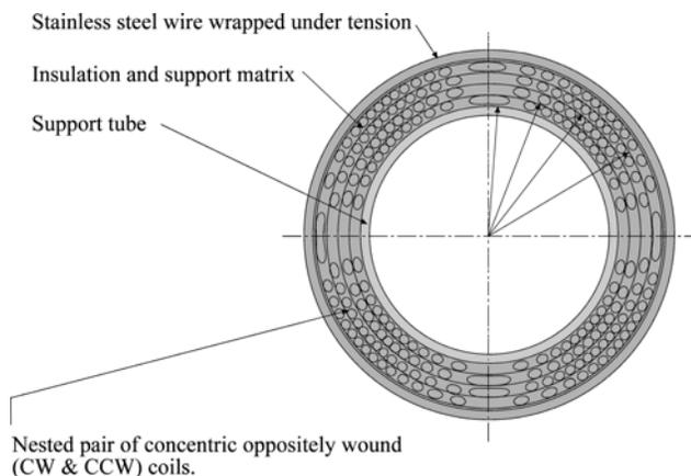
Fig. 6. 130 T/m gradient quadrupole example.
