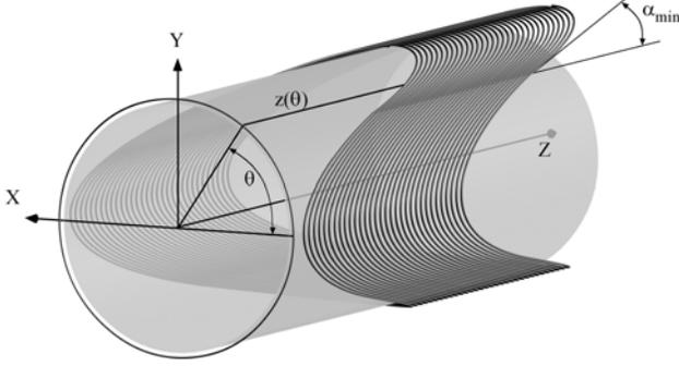
Fig. 3. Helical turns modulated with sine  $2\theta$ .
