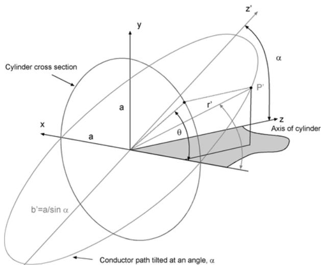
Fig. 1. Coordinates of a tilted elliptical loop.
